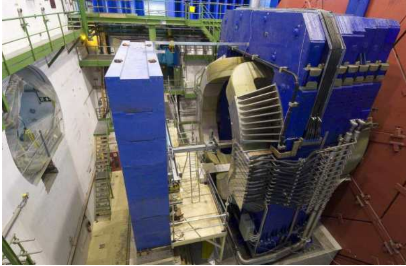
Figure 2.8: The Dipole Magnet of the Muon Spectrometer.
