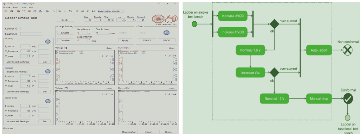
Figure 5.9: Visualisation of the GUI based software (left) and activity diagram (right) for smoke test [8].
