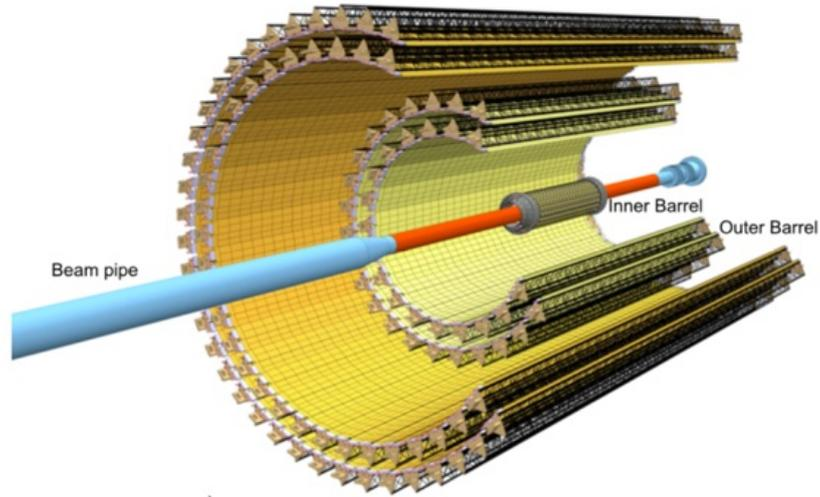
Figure 2.3: Layout of the ITS detector of ALICE [6]
