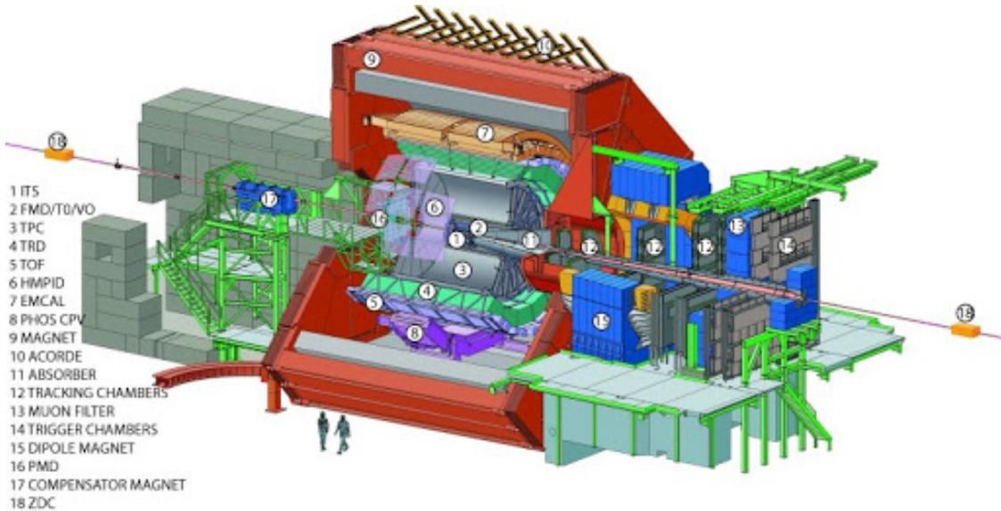
Figure 2.2: Schematic layout of ALICE detectors [2]
