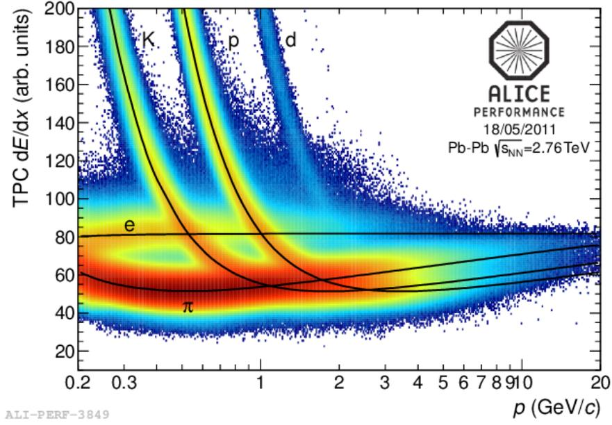
Figure 2.6: Particle Identification using energy loss [15]
