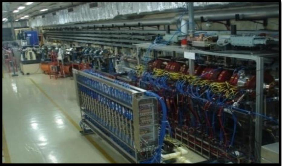
**Infrared Free Electron Laser Developed at RRCAT**
