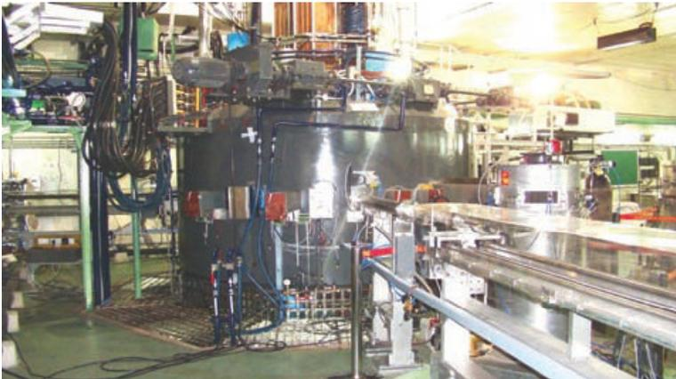
K-500 superconducting cyclotron, under final stages of commissioning.
