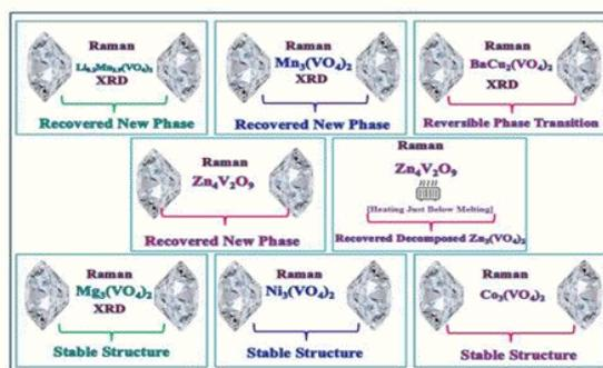
Structural stability of  $A_3(VO_4)_2$  family of compounds ( $Ni_3(VO_4)_2$ ,  $Co_3(VO_4)_2$ ,  $Mg_3(VO_4)_2$ ,  $Li-Mn_3(VO_4)_2$ ,  $Li_{0.2}Mn_{2.9}(VO_4)_2$  and  $BaCu_2(VO_4)_2$ ) and the compound  $Zn_4V_2O_9$
