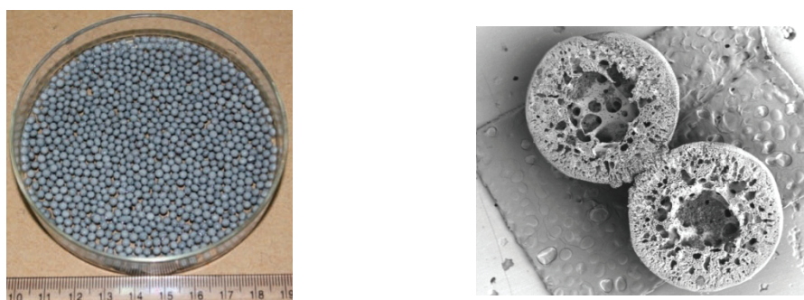
Fig. 2.1.2: Optical and SEM image of PES/MWCNT/D2EHPA polymeric bead
