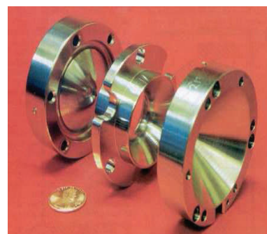
Fig.1.1.7. A quadrupole ion trap for mass-spectrometer
