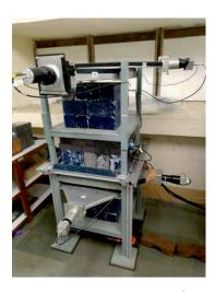
Muon induced neutron measurement setup at TIFR (MINT) has been developed for the measurement of neutrons produced from cosmic muon interactions
