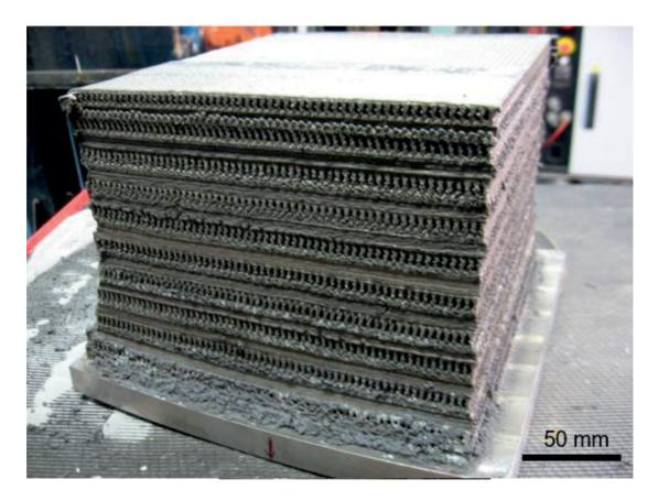
Photographic view of LDED built Printed Circuit Heat Exchanger of size 200 mm x 200 mm x 170 mm.
