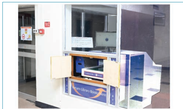
Fig. 2. RFID based book drop system.
