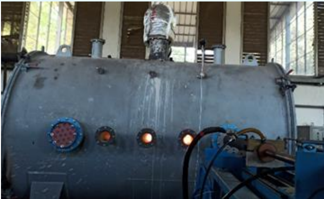
(L) The plasma arc as seen through the viewport (R) Plasma arc using graphite electrodes
